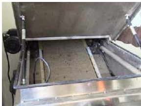
The Salsnes Filter can remove solids as fine as 15-30 microns. The mesh size can be varied depending on the application.
