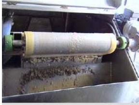
The screen is cleaned as it moves along the conveyor. The solids drop into a hopper. An optional hot water wash cleans grease and oil.
