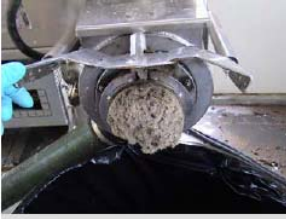
The dewatered screenings will pass the Paint Filter Test. They are generally suitable for land filling; they have also been used as fuel for cogeneration.
